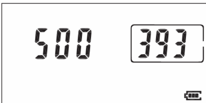
Example 2: Trailer ID (500393) and a flashing trailer.
