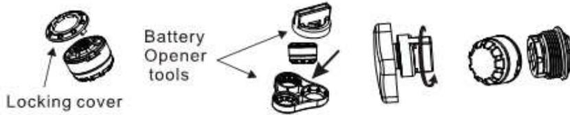
(2) remove battery from battery holder.
