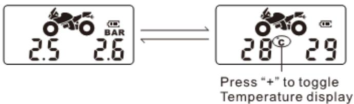
Press the CODE/+ Button to display Temperature
