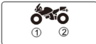
Each sensor has been marked with a sticker has a battery installed and already programmed to the monitor. Install sensors in positions above 1 front wheel 2 back wheel. Sensors can be recoded if the position is changed or a replacement sensor is
