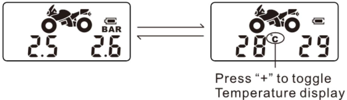
Under normal conditions the monitor will display Pressure for both wheels. To view both tire temperatures press the CODE/+ button the temperatures will be displayed for 10 seconds then resume to pressure display.
