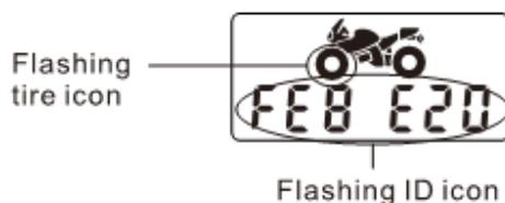
Determine which wheel has the sensor to be replaced. Go to that wheel's tire valve and screw the replacement sensor on the tire valve. The new sensor will transmit its own unique 6 digit code and that will appear on the monitor with a beep sound. To finish and
