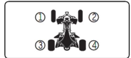
Each sensor has been marked with a sticker and already programmed to the monitor. Install sensors in positions above 1 L front wheel 2 R front wheel 3 L rear wheel, 4 R rear wheel. Sensors can be recoded if the position is changed or a replacement sensor is needed.
