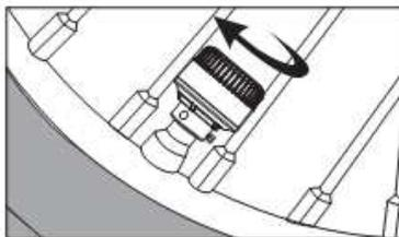
**\*Do not over tighten the sensor cap to prevent possible damage to the sensor.**
